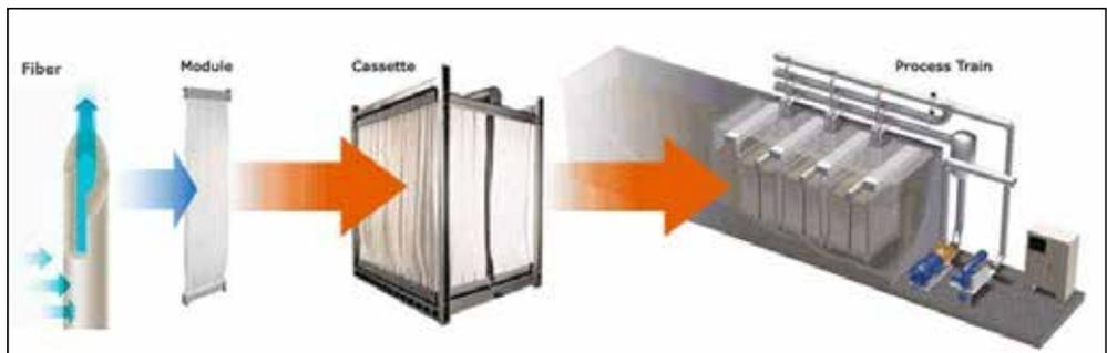
Figure 13. Building Block Design of an Immersed Ultrafiltration Membrane System (courtesy of Suez [Formerly GE], 2016)
